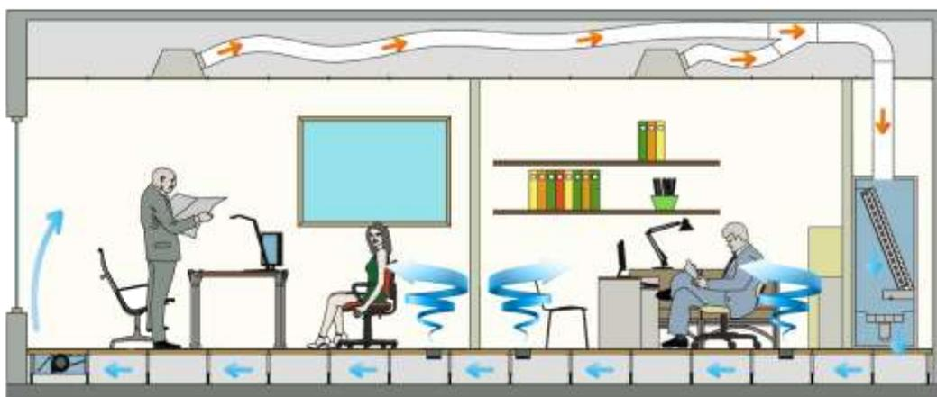
Figure 17 - UFAD system with treated air from an Air Handling Unit with ducted air recovery, floor diffusers in the internal zone and fan-coil in the perimeter
