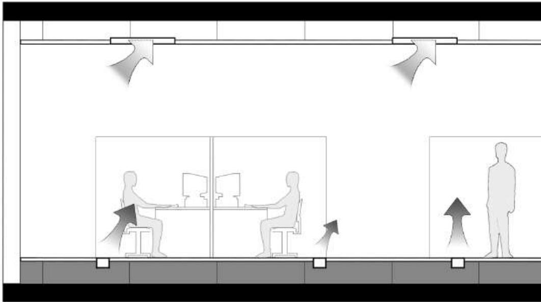
**Figure 4 - Underfloor air distribution system**
