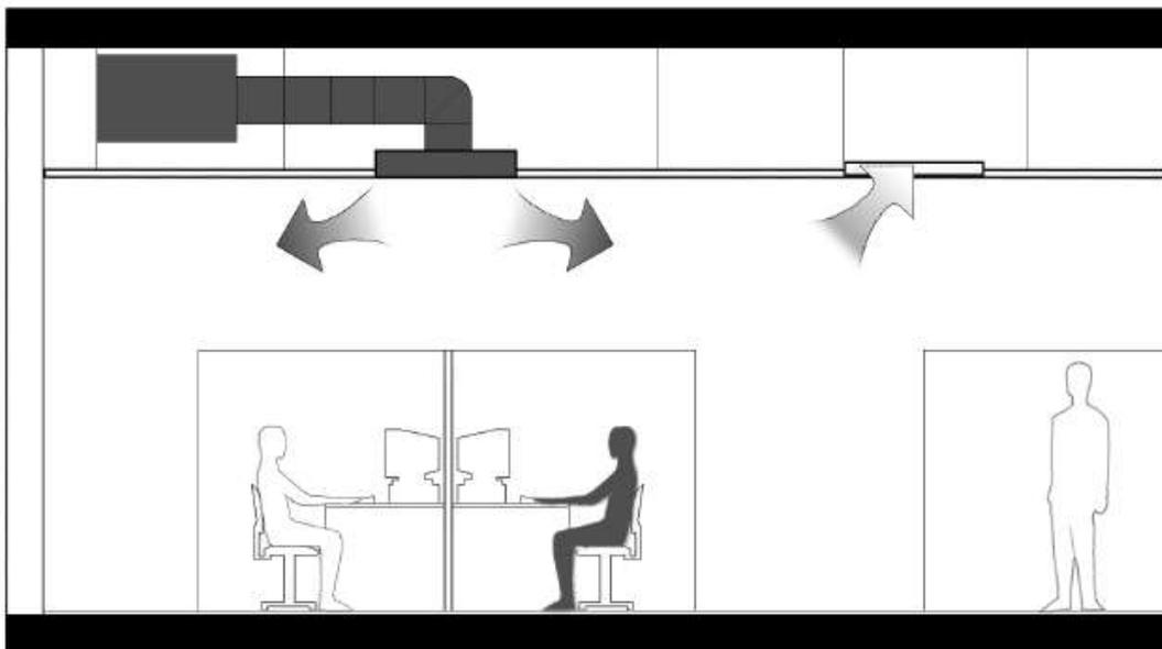
Figure 3 - Conventional overhead air distribution system
