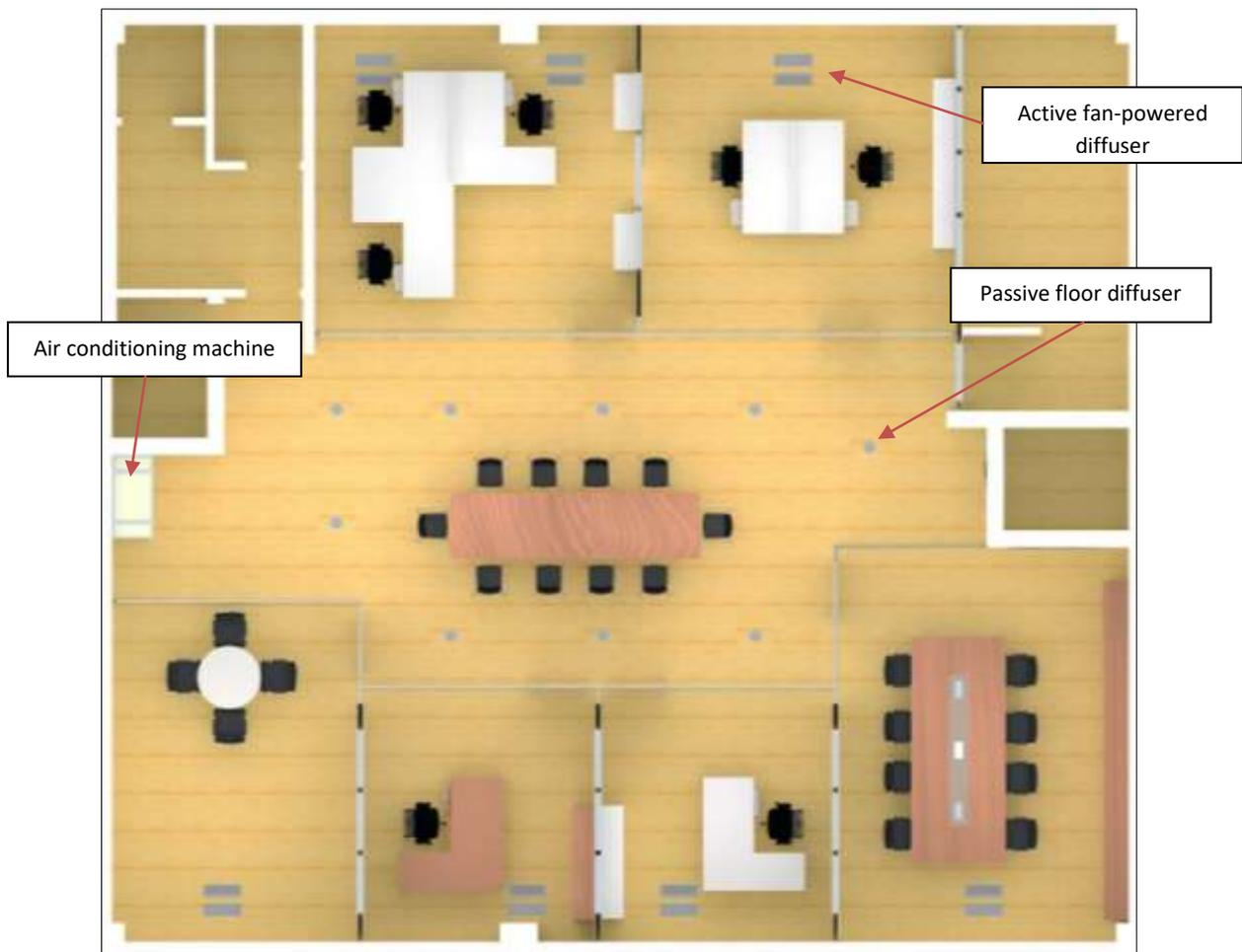
Figure 1 - Example of office with UFAD system. In the interior zone are placed passive floor diffusers, while into the office active fan-powered diffusers are placed to control the temperature singularly.
