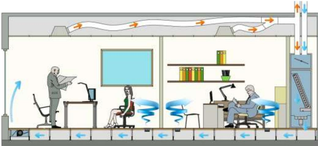
Figure 15 – UFAD system with treated air from an Air Handling Unit with partial renew of the air, floor diffusers in the internal zone and fan-coil in the perimeter
