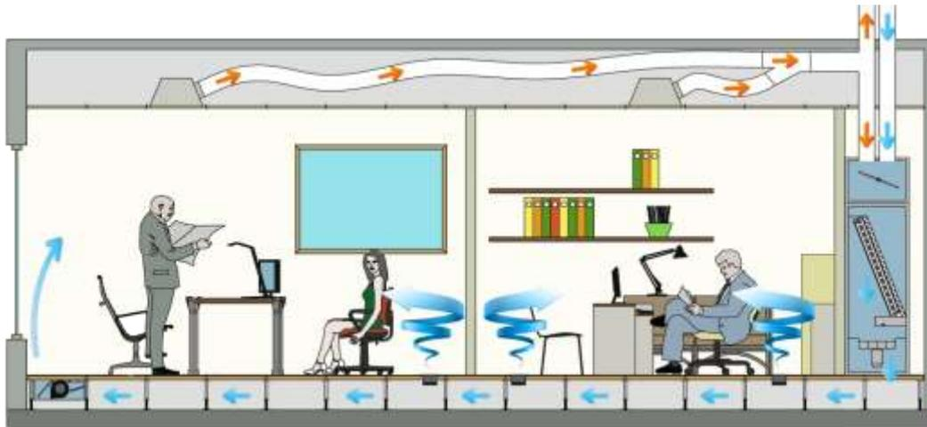
Figure 15 – UFAD system with treated air from an Air Handling Unit with partial renew of the air, floor diffusers in the internal zone and fan-coil in the perimeter
