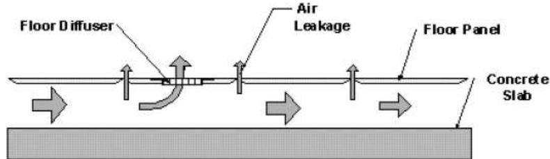
Figure 18 - Airflow and leakage in a pressurized underfloor air supply plenum
