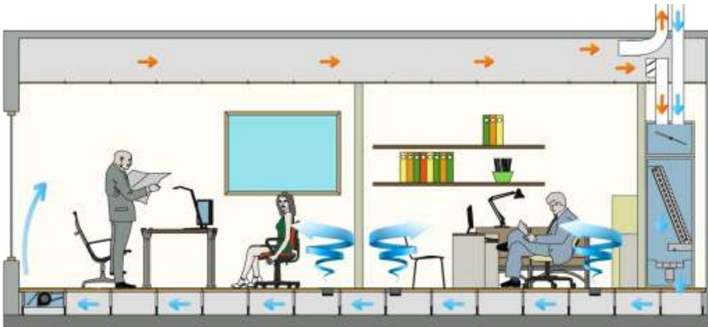
Figure 16 - UFAD system with treated air from an Air Handling Unit with partial renew of air and ceiling plenum no-ducted, floor diffusers in the internal zone and fan-coil in the perimeter
