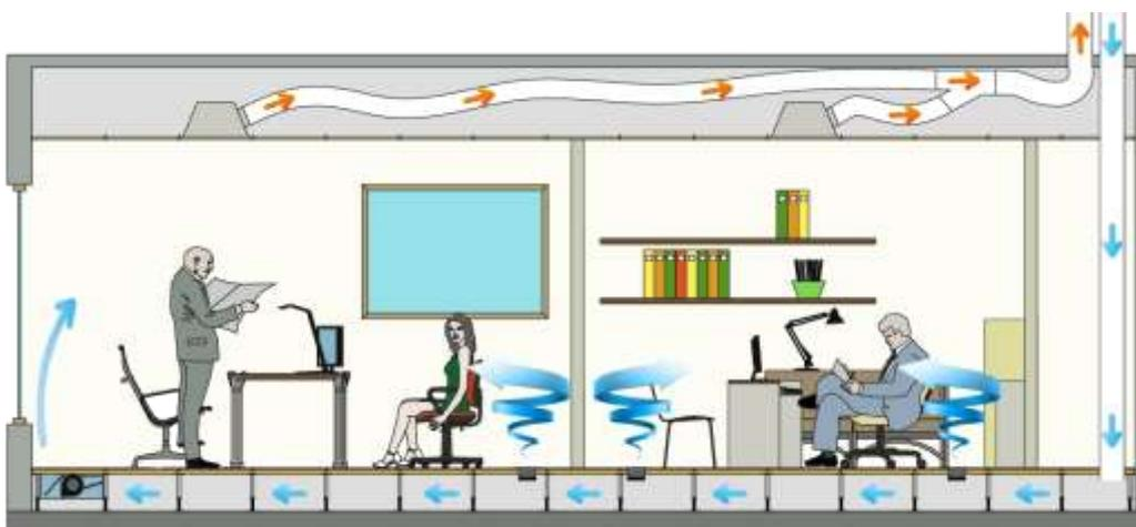
**Figure 14 - UFAD system with treated air from a central Air Handling Unit, floor diffusers in the internal zone and fan-coil in the perimeter**
